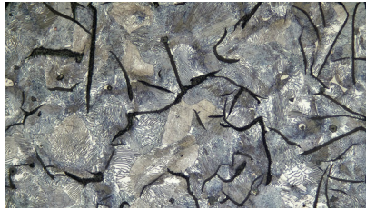
Grey Cast iron (objective: 50X)
