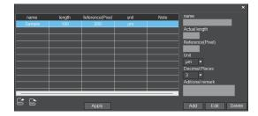
Step 3: When using the mouse to draw a straight line on the micrometer image and setting the scale length, selecting a longer scale length will give more accurate results. For example, selecting 10 small scale lengths will give you more accuracy than selecting only 1 scale length. After releasing the mouse, the image value of the line drawn with the mouse will be automatically updated in the "Benchmark" of the calibration table, as shown in the following figure.
